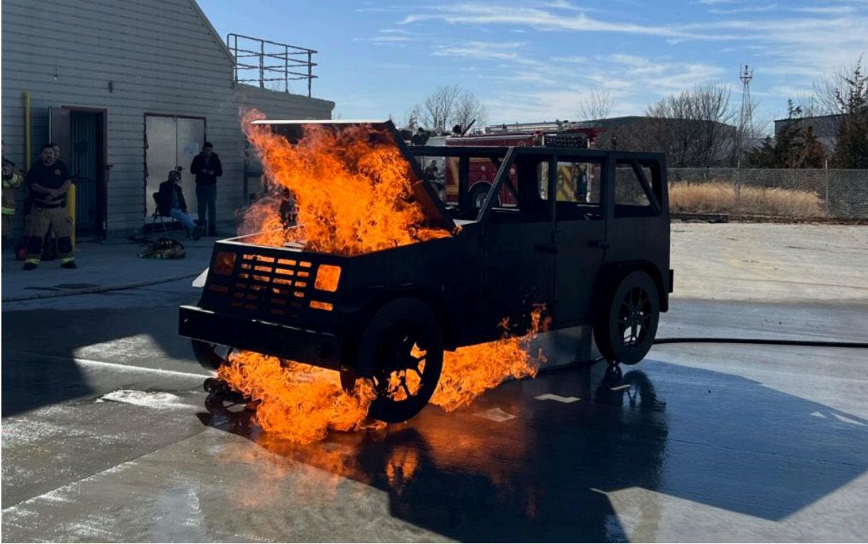
ITEM # 2 – EXAMPLE PHOTO - SUV VEHICLE FIRE TRAINING SIMULATOR MODEL: SYMTECH SUV FIRE SIMULATOR ST+, AS SPECIFIED, OR EQUAL
